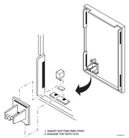
Figure 1. Tamper Magnet Installation
